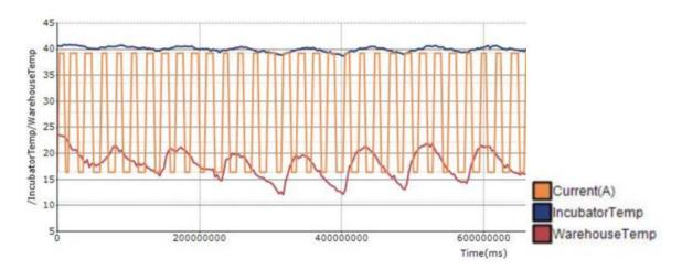
Sample data zoomed out over many days, showing the Any-Cell at 40 ±3 °C chamber temperature while warehouse temperature fluctuates day by day
