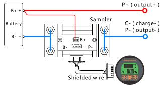
**Attention:** Please connect as shown strictly. The sampler must be connected to the negative circuit, it is forbidden to connect to the positive circuit. If you want to extend the shielded wire, you must use 4 lines of same specification.
